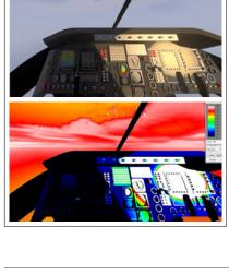
addressing such potential lighting issues as glare, reflection and display washout Simulate ambient lighting parameters
